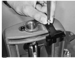
1 INSTALL primer feed bracket with supplied 10-24 screws.
