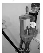
8 LOWER ram (raise handle) to seat the primers. The primers should be flush to slightly below flush when properly seated.
