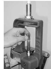
8 BULLET SEATING Adjust the BULLET SEATING DIE per the instructions included with your die. Place a bullet on the case mouth and guide it into the die. Raise the ram to the top and withdraw. The knurled adjusting screw controls the bullet seating depth. Adjust to suit. Usually, seating to the same depth as a factory round works fine. If you desire to crimp, be sure the bullet crimp groove is almost com-
