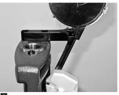
2 INSTALL correct primer feed assembly LARGE white trigger assembly SMALL black trigger assembly into primer feed bracket.
