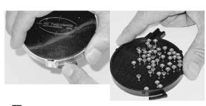
4 DEPRESS primer latch on tray, rotate counterclockwise and lift off cover. Place no more than 100 primers in tray; shake side to side to tip primers upright.
