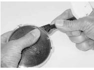
3 LOWER ram and remove primer feed. Remove primer tray from trough.
