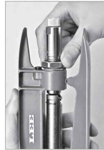
⑧ INSERT a Breech Lock bushing and screw the bullet seating die in until it touches the shell holder and back out one full turn. Fine adjustment will be covered in the next step.
