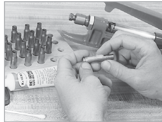
③ PREPARE YOUR CASES Inspect your cases while lubricating them. Discard all cases with split necks, indications of head separation or other defects. Wipe on a thin film of Lee Case Lubricant with your fingers. Fingers are the best way of lubing a case as any grit that could damage the die is wiped away. The case may be immediately sized or you can let the lube dry.
