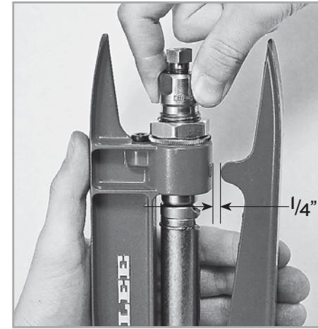
② INSTALL SIZING DIE Insert a Breech Lock bushing and screw the sizing die in until it touches the shell holder and moves the lever off the stop \frac{1}{4} ". When properly positioned, tighten the lock ring. NOTE: DO NOT move the lever off the stop when using carbide dies.
